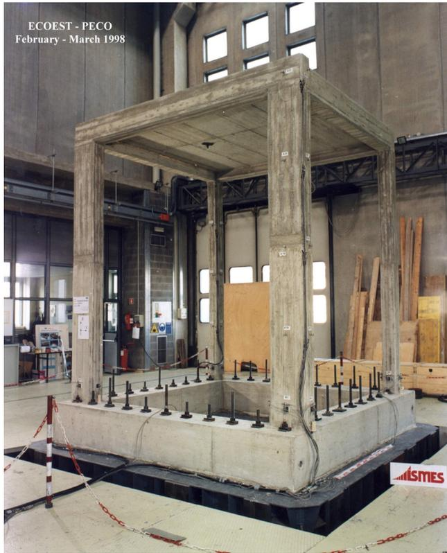
Fig. 1. Photograph showing one of the analysed r/c frames on the shaking table.
